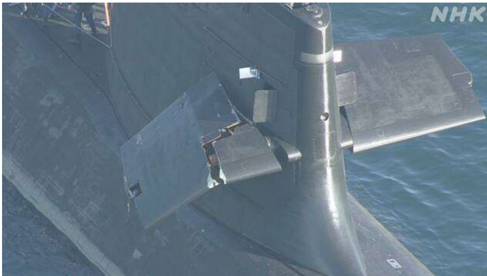
Figure 1: The damaged starboard side diving plane of the Sōryū . Image source: https://www3.nhk.or.jp/news/html/20210209/k10012857021000.html (accessed February 10, 2021)
